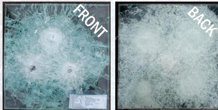
**LEVEL 2 - UL Standard:** Level 2 bullet-resistant glass must withstand 3 shots from a .357 Magnum with jacketed lead soft point bullets.
