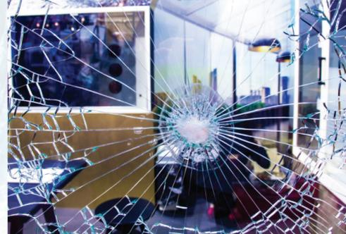
**IMPACT-RESISTANT** glass is two layers of glass with a laminated interlayer designed to slow an intruder's progress. It does not stop bullet penetration but will provide resistance to impact from objects such as rocks and sledgehammers. This will protect, for a time, property in the event of specific glass shattering impacts. This will not provide bullet resistance.
