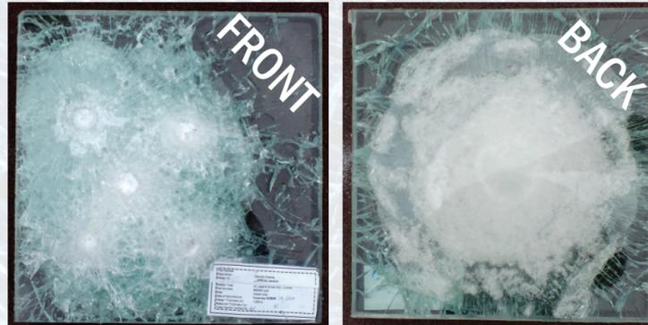
**LEVEL 6 - UL Standard:** Level 6 bullet-resistant glass must withstand 5 shots from a 9mm with full metal copper jacket with lead core ammunition.
