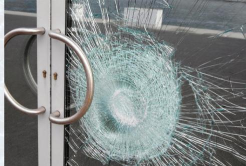
**SAFETY-GLASS** is two layers of glass with Polyvinyl Butyral (PVB) or Security Guard (SGP) in the middle. It is designed to protect from unintentional impacts.
