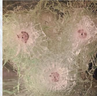
**BULLET-RESISTANT** glass is made with multiple layers of laminated glass and is designed to displace the energy of ballistic rounds like those of handguns, assault rifles and automatic weapons, flattening or catching the bullet(s) and preventing them from penetrating. This will offer the highest level of protection to both property and people.
