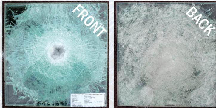
**LEVEL 4-5 - UL Standard:** Level 4-5 bullet-resistant glass must withstand 1 shot from a .30 caliber rifle with lead core ammunition or 1 shot from a 7.62 mm rifle with lead core full metal copper jacket military ball ammunition.
